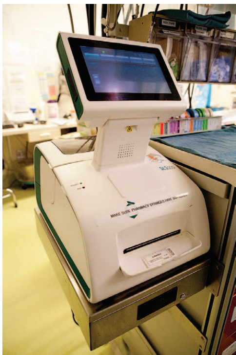
Figure 1. The Codonics SLS drug labeling system mounted on the side of the anesthesia cart.
